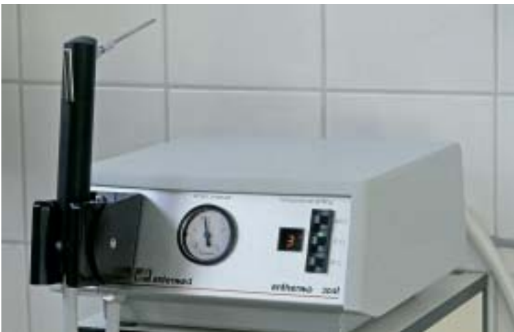
Figure 1.6: An apparatus developed for ear flushing. It consists of a small heater in which tap water is warmed to body temperature and held there. The water is sprayed into the ear canal through a short cannula, at the pressure indicated on the display.
